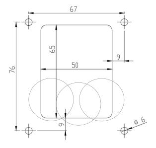
To begin, drill holes in the dispenser panel for the mounting screws as well as cutting out the area for the cables to pass through (this may be possible with 3x 25mm holes) as per the diagram left.
