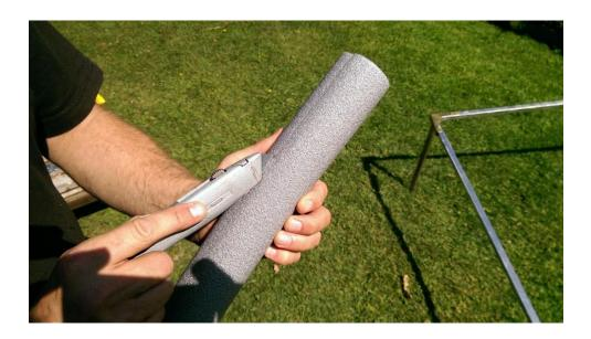
Wrap the lagging around the diamond shaped frame, taking care to get the corners as tight as possible, place cable ties (J) around the perimeter to hold the lagging firmly to the frame
